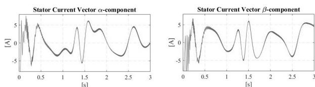
Fig. 2. ( $\alpha$ ,  $\beta$ ) components of stator current vectors.
