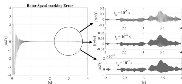
Fig. 4. Rotor speed tracking error for different sample times.
