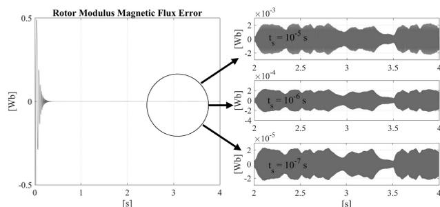
Fig. 5. Flux modulus tracking error for different sample times.
