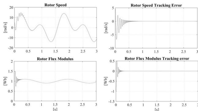
Fig. 1. Rotor speed, flux modulus and corresponding tracking errors.
